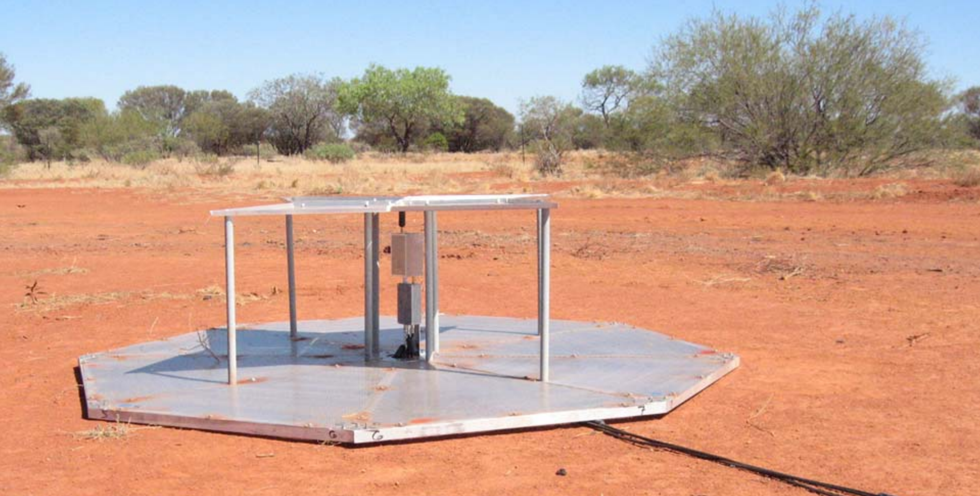
Experiment to Detect the Global EoR Step - EDGES antenna at Mileura WA
