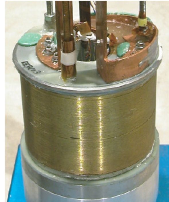
Figure 3. Fabricated GdBCO coil installed in the 17.2 T low-temperature superconducting magnet.
