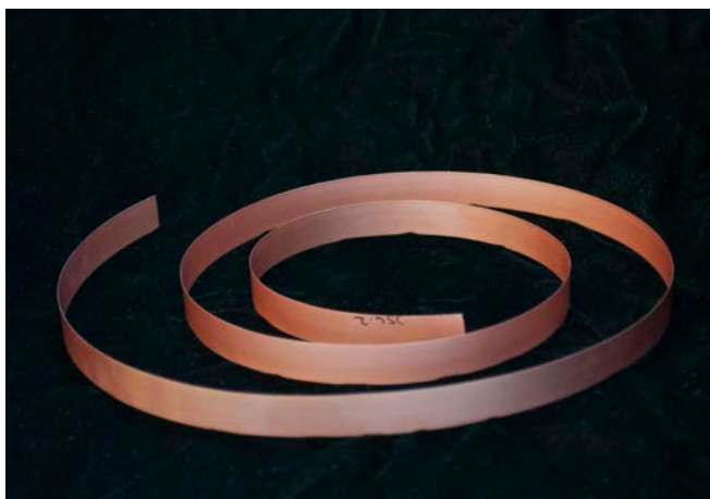
Figure 2.1 REBCO superconductors are available in thin, flexible tapes. The superconducting material is deposited in a thin layer on a strong steel substrate.
