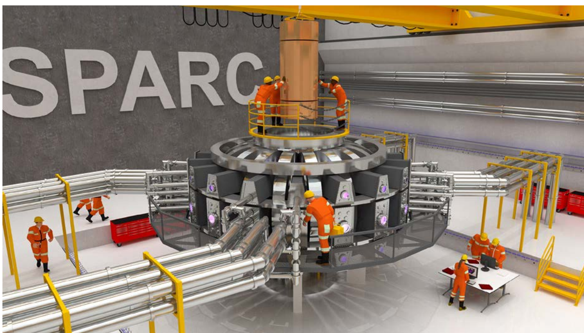
An illustration of the SPARC device as it might appear during construction, showing the coaxial feed lines for 30 MW of ICRF heating. Credit: Ken Filar
