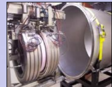
NIST's 0.5 meter Guarded Hot Plate Capable of Providing Measurements of Thermal Insulation from 90 to 900 K
