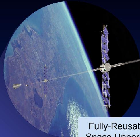
Tether propulsion enables large  $\Delta V$  missions to be performed by re-usable, low mass systems
