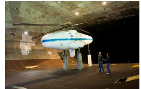
UH-60A Airloads test configuration in the NFAC 40x80ft Wind Tunnel
