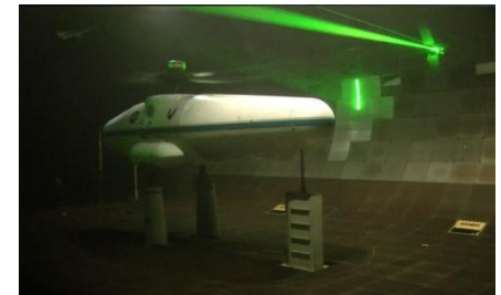
Laser-illuminated flow visualization to image and measure rotor wake velocities
