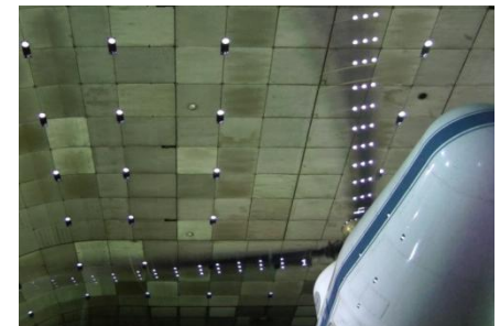
Optical targets for elastic blade bending measurements
