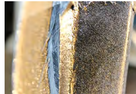
Post-failure pictures of imperfect specimen. Grey/blue zone under flange represents manufacturing defect.
