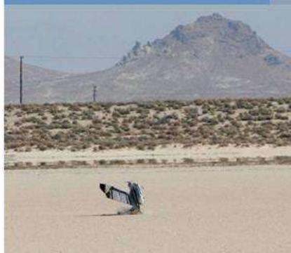
**Left:** Air Force Research Laboratory's Multi-Utility Technology Testbed (MUTT) aircraft, built by Lockheed Martin. This vehicle was designed to test the limits of aircraft structures, including the point where the wings would flutter so much that they would break. The crash is therefore not an accident, but the end result of the test. This kind of flight research cannot be conducted with piloted vehicles. (Source: Jeff Beranek, Lockheed Martin.)
