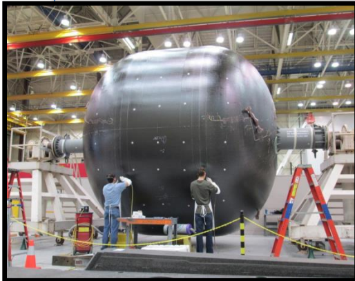
Top Image shows STMD management with the 5.5 meter diameter composite tank test article. Bottom images side view of tank and (right) shows the placement of fibers onto the 5.5 meter diameter tank.
