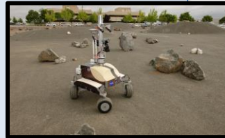
Top Image: K10 Rover on Lunar roverscape being controlled by astronaut on the ISS Left Image: Robonaut 2 (R2) is the first humanoid robot in space. The robot can work with the same hand tools and hardware (switches, connectors, etc.) as used by astronauts.
