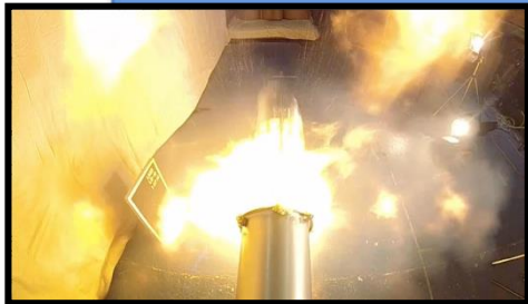
Successful test firing of Ballute mortar (used to deploy supersonic parachute)
