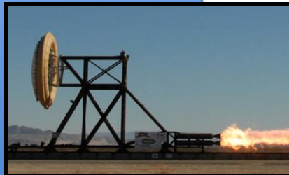
Rocket sled testing of robotics- class supersonic decelerator
