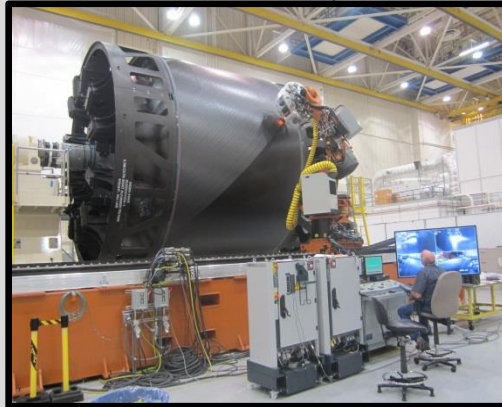
Top Image shows STMD management with the 5.5 meter diameter composite tank test article. Bottom images side view of tank and (right) shows the placement of fibers onto the 5.5 meter diameter tank.
