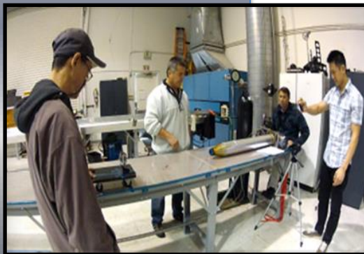
Engineering Development Unit Solar Sail quadrant deployed during ground demonstration
