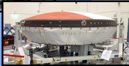
Integration of Supersonic Inflatable Aerodynamic Decelerator (SIAD) onto first flight demonstration vehicle; Top , inflated for dimensional verification; Middle , deflated, being packaged; Bottom , completed packaging
