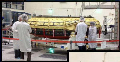
Integration of Supersonic Inflatable Aerodynamic Decelerator (SIAD) onto first flight demonstration vehicle; Top , inflated for dimensional verification; Middle , deflated, being packaged; Bottom , completed packaging
