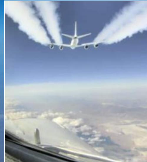
NASA Falcon Aircraft in Flight Behind DC-8 Aircraft
