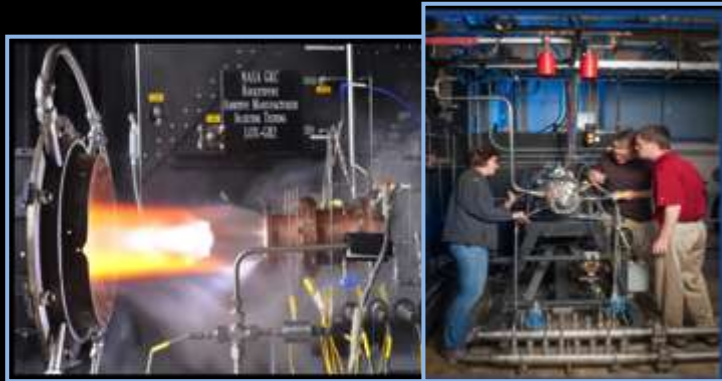
Additive Manufacturing for combustion chambers and nozzles
