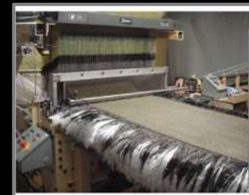
3-D, multi-layer preform weaving technology for thermal protection
