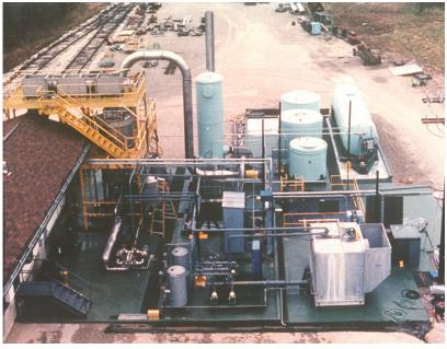
The APE 1400 Phosphoric Acid Conversion plant consists of two systems: feed system acid plant conversion system.
