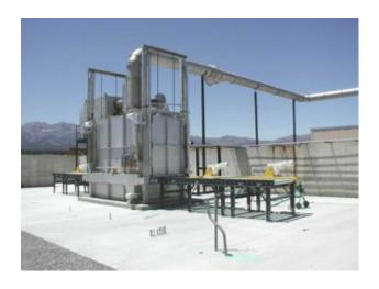
The APE 2048 Flashing Furnace System is used to remove residual explosives from metal components, removing residual energetics to allow safe sale of scrap metal to the general public. It can be used as part of a "R3" facility to decontaminate processed munitions (105mm Cartridges to 750 pound bombs). It is not used to flash explosively contaminated waste.
