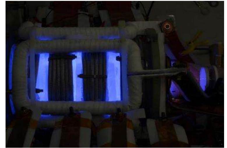
MSNW: Electrodeless Lorentz Force plasma thruster.
