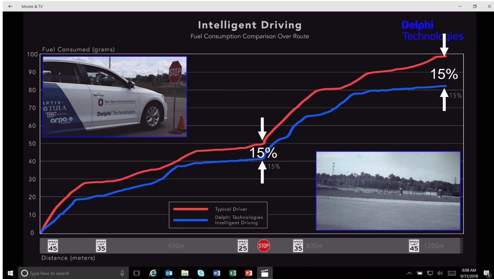
Fuel Consumption Evaluation on Test Track with NEXTCAR Development Vehicle
