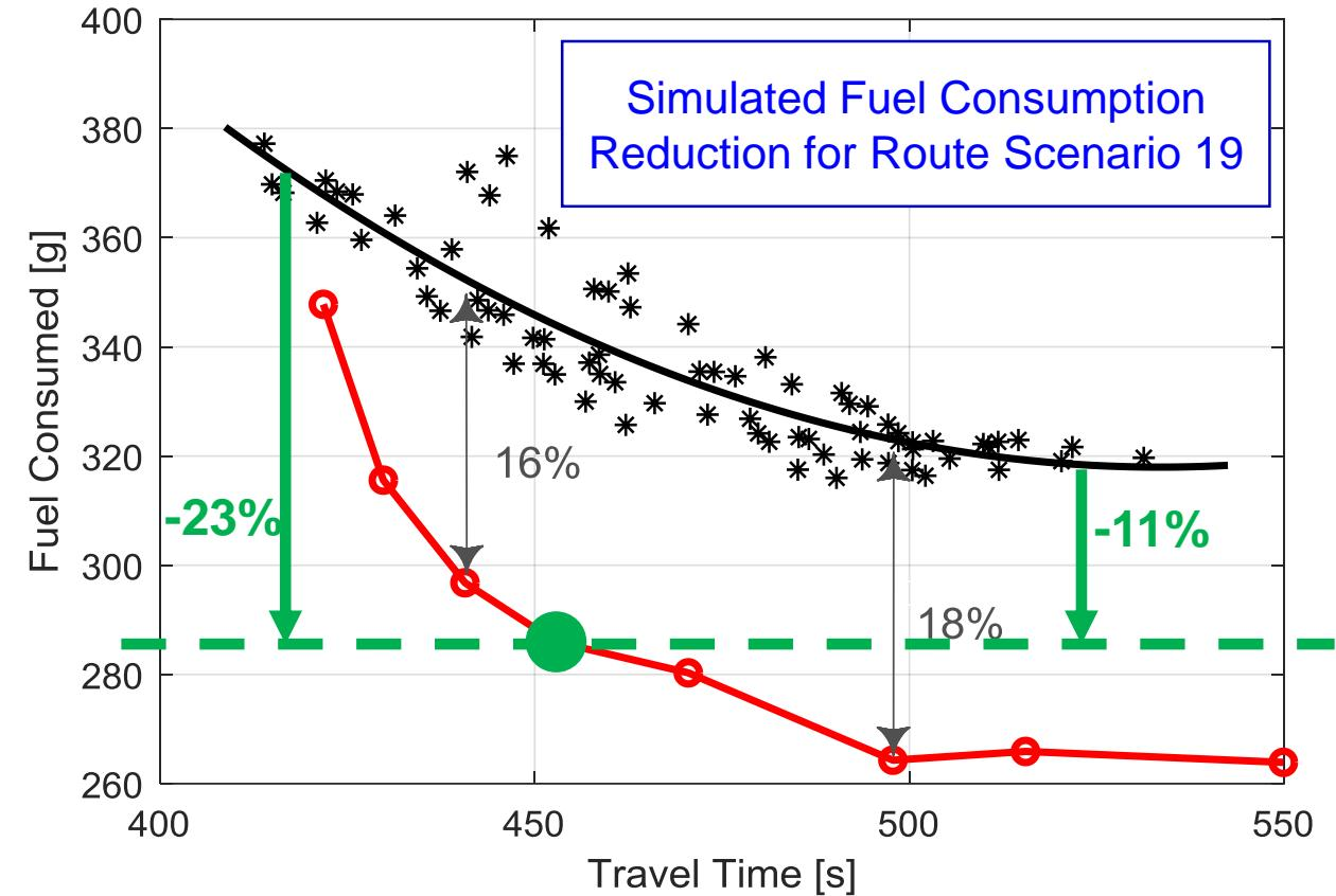
Simulated Intelligent Driving Controls Demonstrate Significant Potential Benefit
