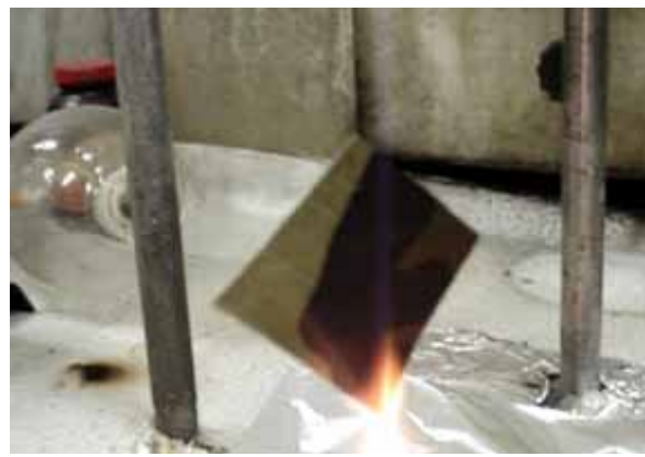
Laboratory burning test of Army's camouflage fabric sample
