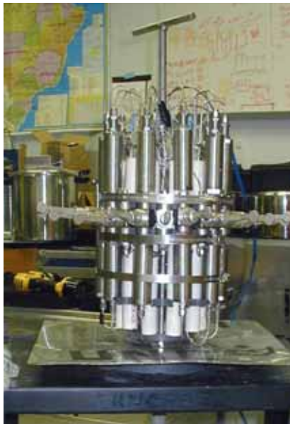
Figure 2: The first pore-water probe with high pressure stainless steel sample chambers and on/off valves. The 50-cm probe tip is visible below the lab cart. Inserting the probe into the sediment required the entire device to be manipulated on the seafloor.
