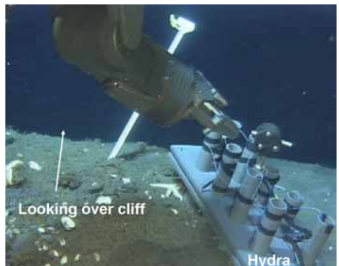
Figure 4: A second generation adaptation showing the decoupled probe tip (A) being manipulated by a submersible robot arm and inserted into sediments beneath a mussel bed.
