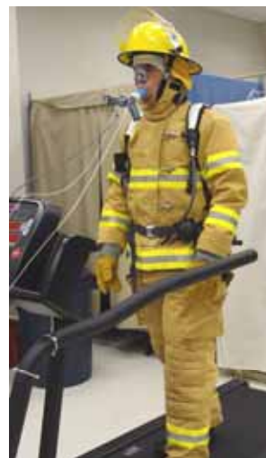
Dr. Coca simulating a laboratory test wearing a firefighter ensemble
