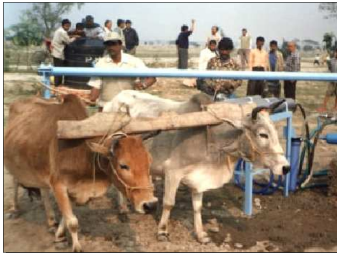
Oxen-driven water pump equipped with nanofilters in India
