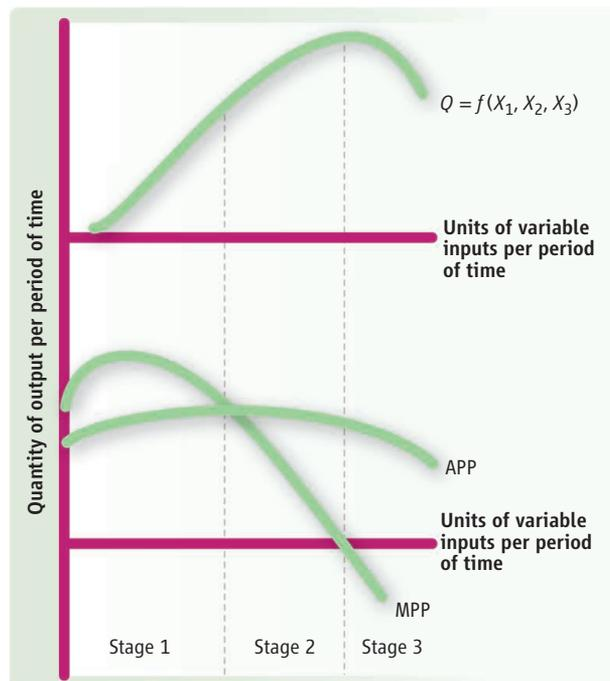
**A standard approach to linking inputs and outputs that has been used to study innovation.** Output ( $Q$ ) is shown as a linearizable function of inputs ( $X_1$ ,  $X_2$ , and  $X_3$ ). The efficiency of different stages of production is described by the relationship between average physical product (APP) and marginal physical product (MPP).
