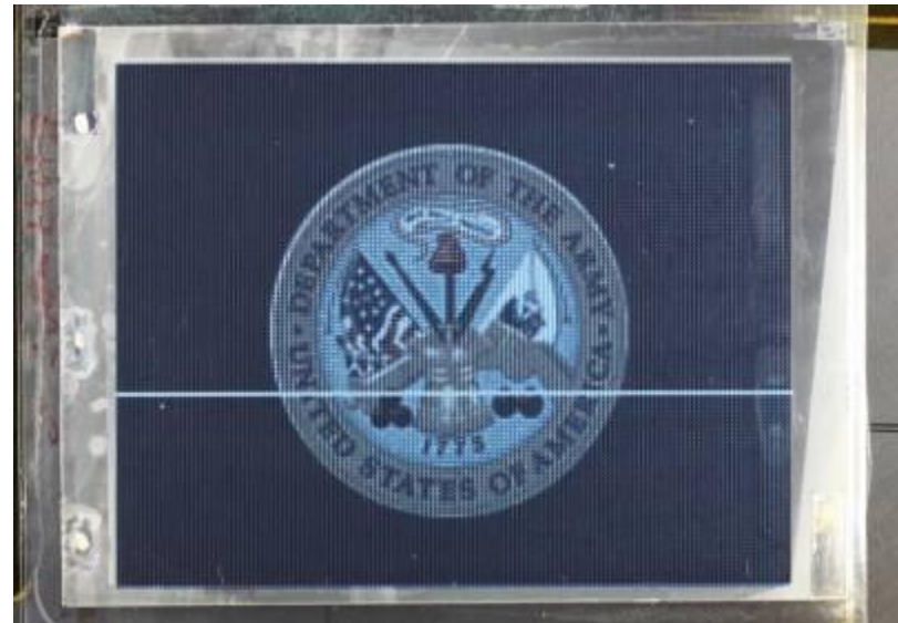
Templated color filter array laminated to FCD E-Ink display
