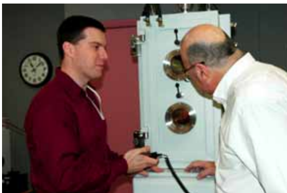
Left: NRC Associate, Dr. Neil Baril, and NRC Adviser, Dr. Joe Pellegrino, looking at a thermal evaporator used to deposit thin films for passivation
