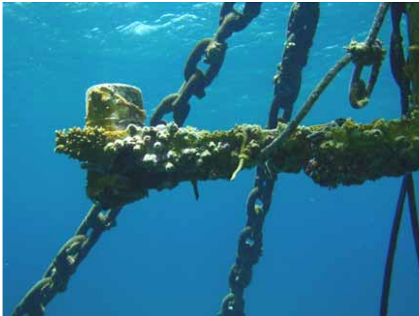
Barnacles and other marine growth are visible on the support chains that anchor the St. Croix station to the ocean floor, as well as on one of the subsurface instruments.
