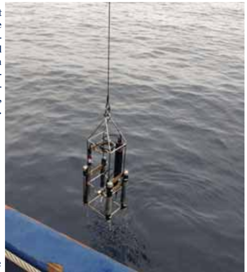
Figure 1: Deployment of the ADV package of the UNOLS research vessel R/V New Horizon in the California Borderlands on November 15 under ideal, calm conditions.
