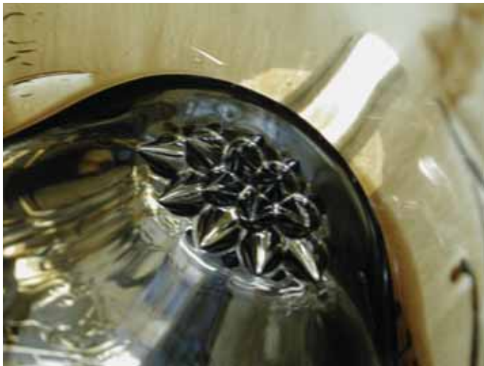
Figure 2 Visualizing the magnetic field of a neodymium rare-earth magnet with a ferrofluid. Photo by Peter Hsieh.
