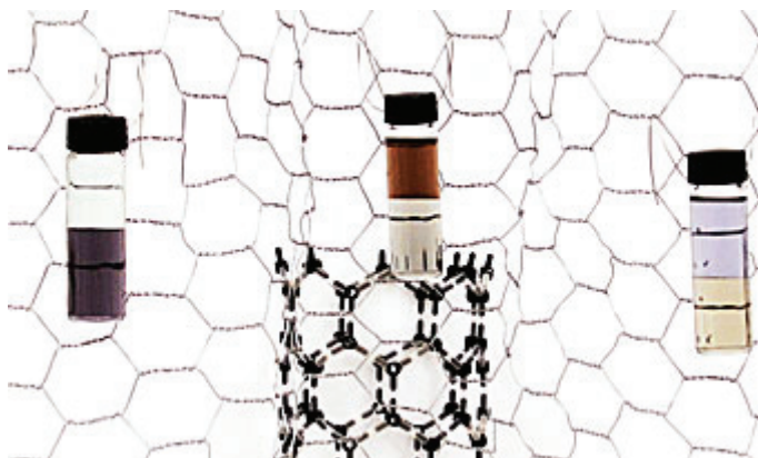
Three examples of partitioning carbon nanotubes in liquid phases. Left: nanotubes partitioned by diameter. Smaller diameters, on the bottom, appear purple. Center: partitioned between semiconductors (amber, top) and metals. Right: A sample with different diameter range partitioned between metals (yellow) and semiconductors. Color differences are due to differences in electronic structure.
