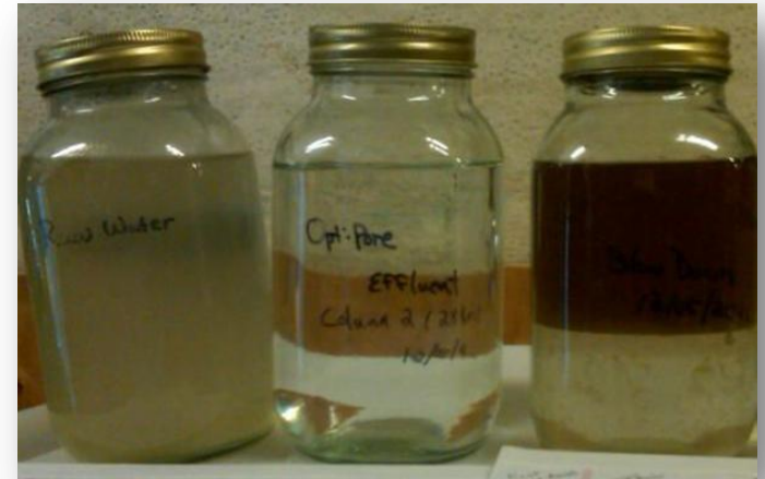
DOWEX OPTIPORE BTEX removal and recovery system demonstration: Raw Water (left), Clean effluent (middle) & Recovered Condensate (right)
