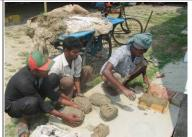
Molding of semi solid mass for bricks preparation
