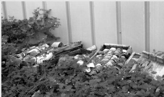
Cores stored outside at Oakridge National Laboratory, Tennessee, in Spring 2001. These cores are from the Tennessee Valley Authority's Clinch River Breeder Reactor site. Rescue of cores in this state of degradation is unlikely given the probable loss of documentation associated with them. SOURCE: Richard Pawlowicz, Bechtel National, Inc., San Diego, California.
