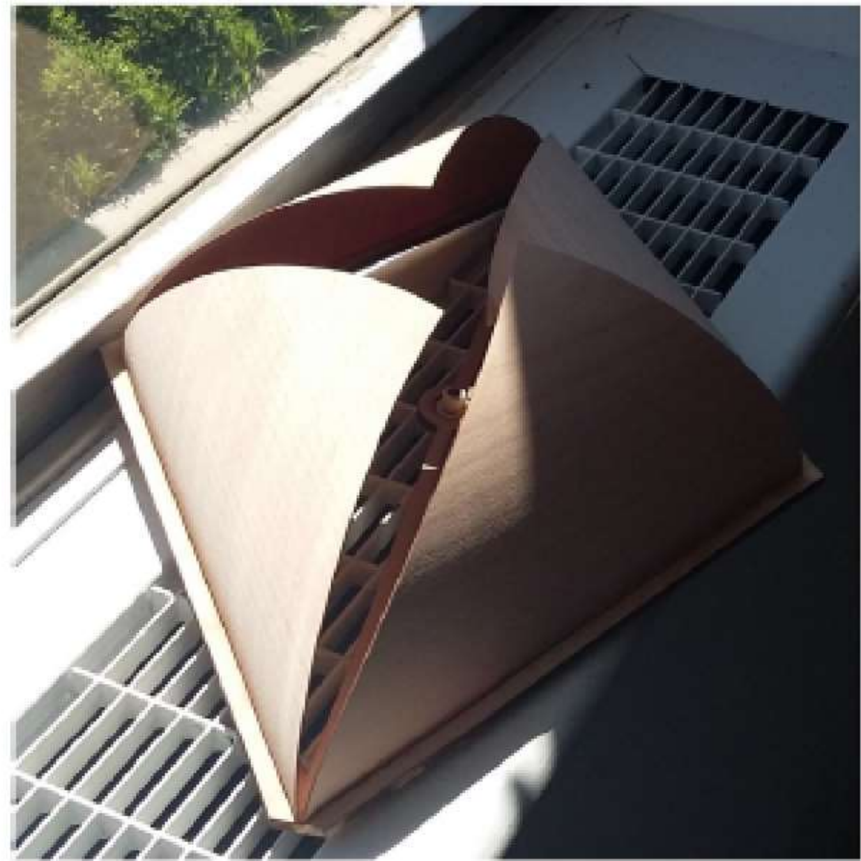
Physical implementation of the diamond module – simulation of the closure.
