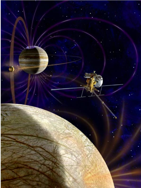
**Figure ES-4. The JEO flight system would use radioisotope power and deliver a complement of 11 instruments to explore Europa and the Jupiter System.**
