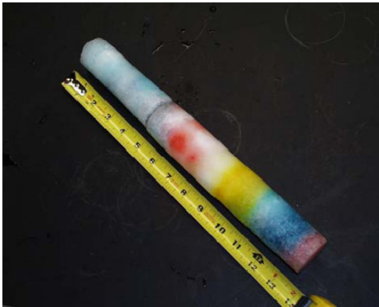
Figure 6-10. Ice core sample showing stratigraphy from a comet core sampler. (Image reproduced from ref. 11.)
