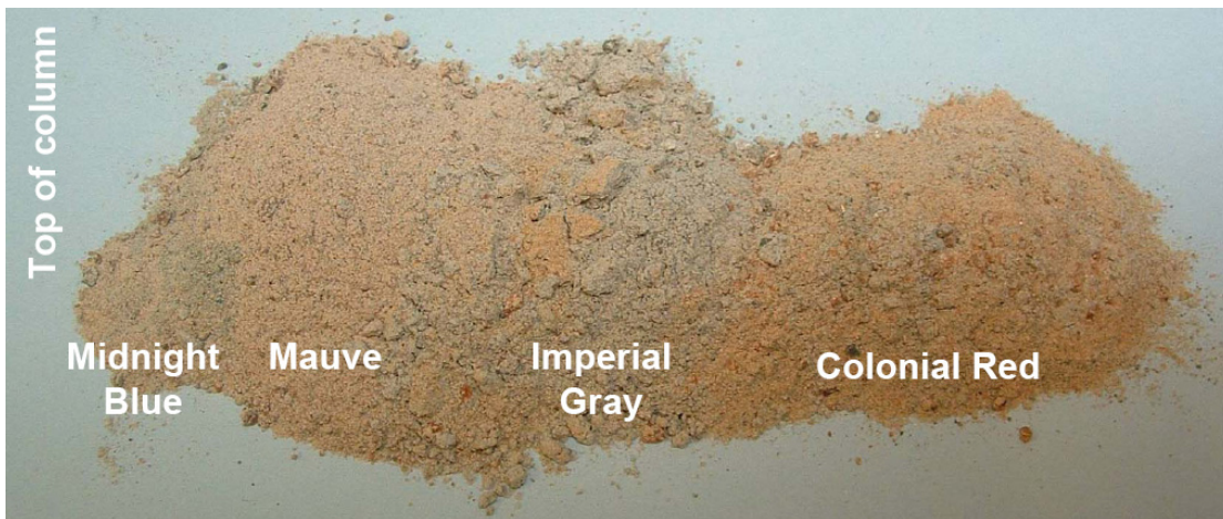
Figure 6-12. Regolith core sample, as poured from the sample in Figure 6-11, showing that stratigraphy was maintained following a re-entry simulation. (Image reproduced from ref. 13.)
