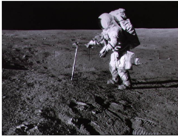
Figure 2-1. Astronaut Alan Bean driving a core sampler into the lunar surface with a hammer. (Image courtesy of the NASA JSC Imagery Services, http://science.ksc.nasa.gov/mirrors/images/html/as12.htm .)
