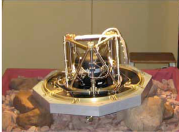
Figure 3-1. SEIS showing the evacuated sphere where the VBB sensors are located, the base, and support structure.
