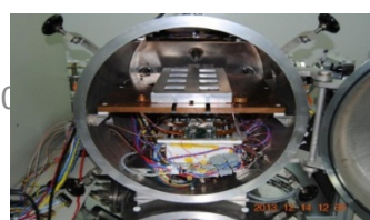
The electronic box (left) and one detector box of LE in environment tests.
