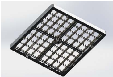
Design of one MPO lobster-eye telescope optics module
