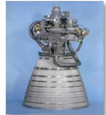
RL10 Sheet Metal + Welded Inlets now SLM
