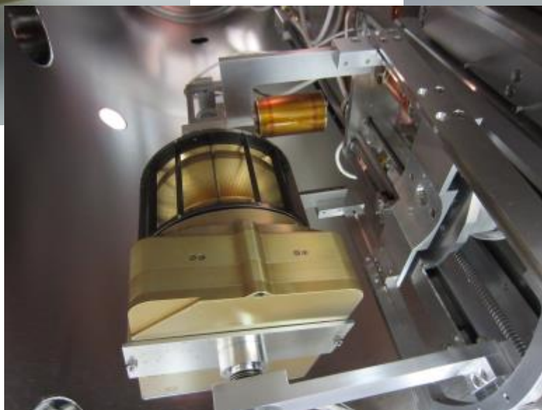
SWEAP SPAN-Ae FM Goes Into the Calibration Chamber
