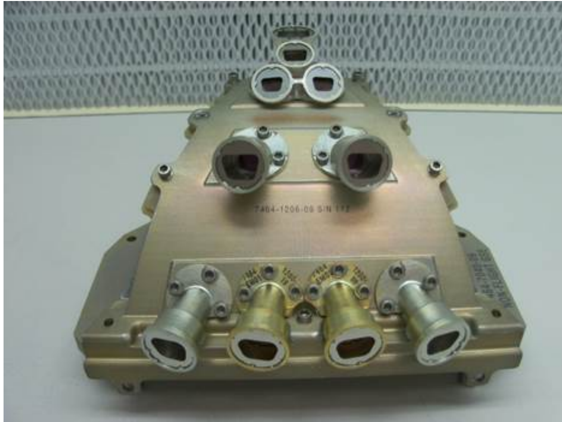
ISOIS EPI-Lo FM Wedge Assembly Complete Undergoing Vacuum Testing with Sources
