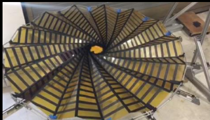
Positioning the petals to high precision, blocking on-axis starlight, maintaining overall shape on a highly stable structure
