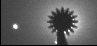
Suppressing scattered light off petal edges from off-axis Sunlight
