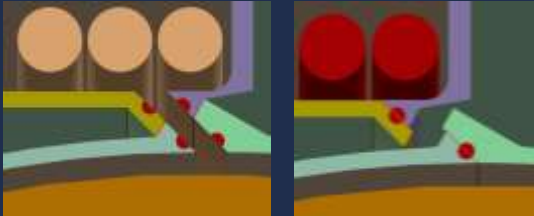
Sealing via in-flight brazing (Simultaneous heat sterilization)
