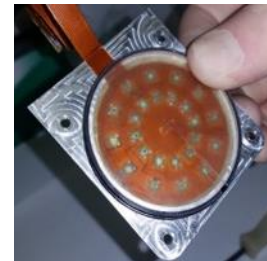
BRIC-LED PDFU Lid showing LEDs.
