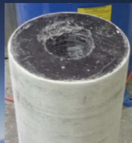
Paraffin Motor "Grain" Casting
