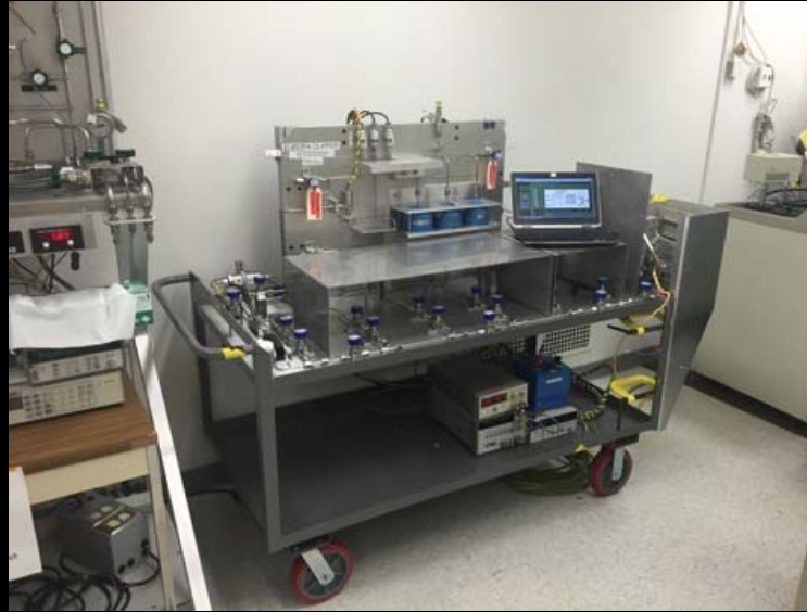
Thermal Pump Life Test (Irradiated CFC-11)
