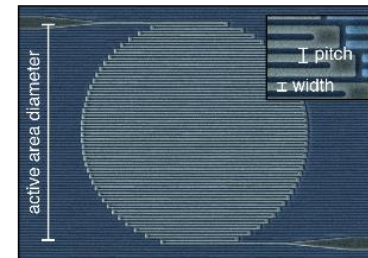
Electron microscope detail of 320 \mu\text{m} active area tungsten silicide (WSi) superconducting nanowire single photon detector (SNSPD) array
