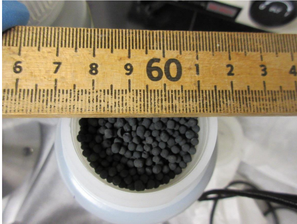
Packed bed material for ISS WRS, Catalytic Oxidation Reactor (Alumina or Zirconium beads)
