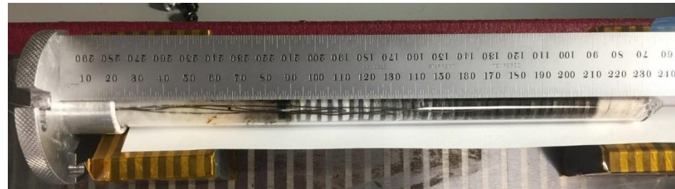
SUBSA furnace sample test ampoule is shown above. It is a quartz tube which contains aluminum discs, meant to simulate the brazing coupons, separated by alumina cloth. Also included in the quartz tube are 4 thermocouples.
