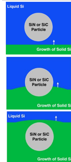
Engulfment of particles during silicon crystal growth
